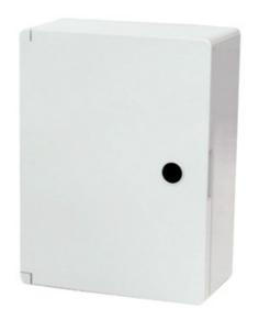
The Termination Technology range of IP65 Watertight Boards are available in a range of sizes to accommodate a wide range of applications. Manufactured from ABS in Grey (RAL 7035) with triangle lock-key. Supplied complete with a 1mm thick adjustable galvanized steel mounting plate and reversible door.
