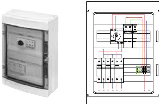
Pre-wired board for connecting 3 strings of photovoltaic panels to the inverter. It includes:
