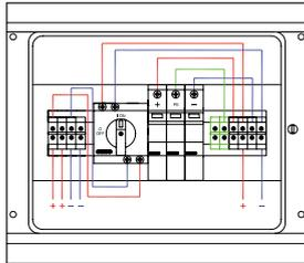
Pre-wired board for connecting 1 or 2 strings of photovoltaic panels to the inverter. It includes:
