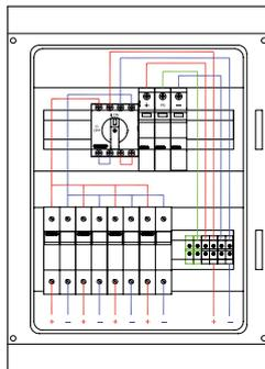
Pre-wired board for connecting 4 strings of photovoltaic panels to the inverter. It includes:
