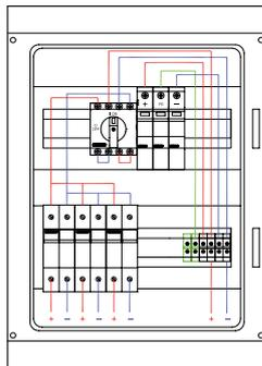
Pre-wired board for connecting 3 strings of photovoltaic panels to the inverter. It includes:
